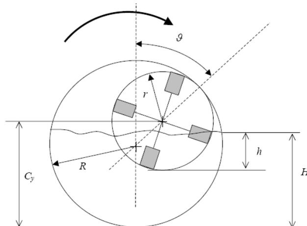
**Figure 4 – Impeller planetary motion**
