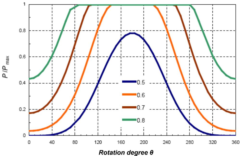
**Figure 5 – Impeller power consumption as per equation (1) during planetary motion versus dryer chamber filling**
